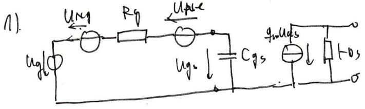
$$2) \underline{C}_{igs} | \underline{C}_{ing} = \frac{j\omega C_{gs} \cdot \underline{U}_{ng}}{R_g + j\omega C_{gs}} = \underline{C}_{ine}$$
