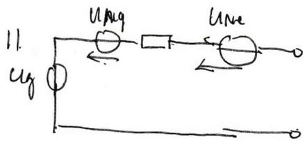
$$2) \underline{S}_{une} = \begin{pmatrix} \underline{G}_1 & \underline{G}_2 \end{pmatrix} \begin{pmatrix} S_{UN} & S_{UI} \\ S_{IU} & S_{IN} \end{pmatrix} \begin{pmatrix} \underline{G}_1^* \\ \underline{G}_2^* \end{pmatrix}$$
