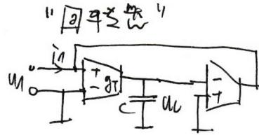
$$U_c = \frac{1}{j\omega C} I_1, \quad i = \frac{dI}{dt} = \frac{CdU}{dt} \Rightarrow I_1 = C \cdot \omega U_c$$
