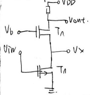
$$\text{对于 } Tn_1: V_x > V_{in} - V_{th1}, \quad V_x = V_b - V_{GS2} \Rightarrow V_b > V_{in} - V_{th1} + U_{GS2}.$$
